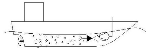
Figure 12 Schematic drawing of an air lubrication system with a compressor and a non return valve
