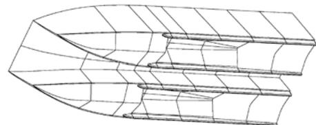
Figure 9 Hull of the air lubrication catamaran model
