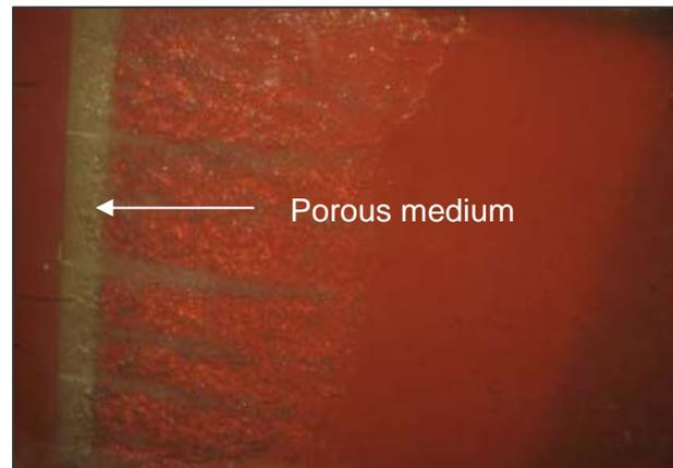
Figure 11 Air bubble layer lubrication
