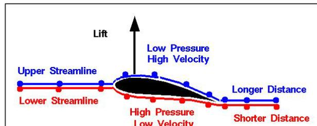
Figure 6 Physics of the propeller blade creating lift
