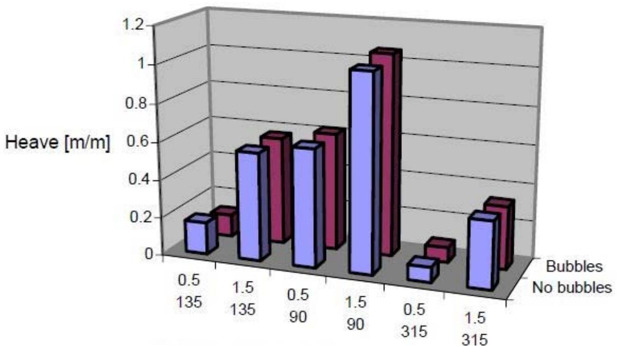
Figure 15 Heave reaction due to wave height and heading
