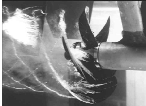
Figure 8 Cavitation occurring on the propeller under water
