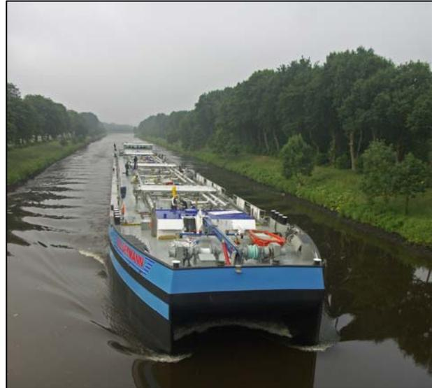
Figure 16 A picture of the Till Deymann, a semi-twinhull bow type ship with air lubrication
