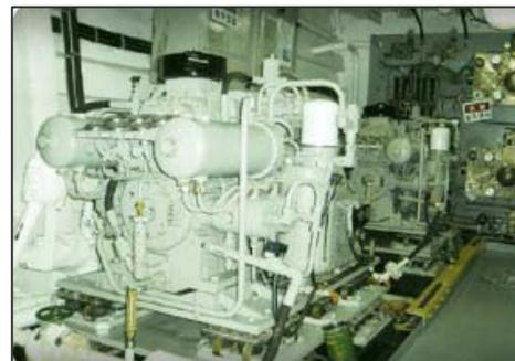
Figure 10 Air-compressor on board a vessel
