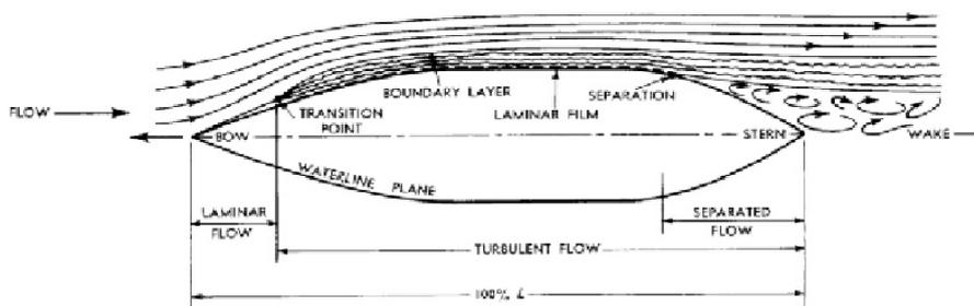
Figure 2 Boundary layer, viscous and pressure drag
