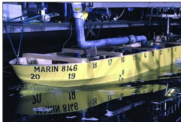
Figure 13 Model in the Marin air lubrication project
