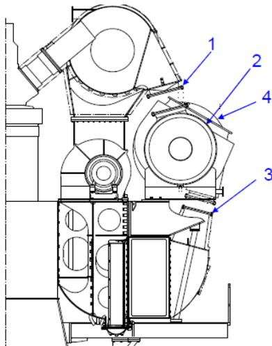
Blinding turbocharger with blanks before removal
